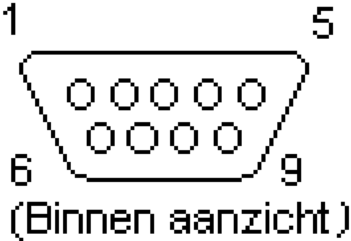
Figure 11.3: Serial-9 pinout view from inside
